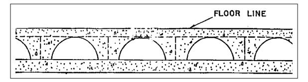
Each Airfloor form displaces 0.223 cu. ft of concrete per sq. ft. One (1) inch of concrete is required to fill the void formed by the corners of the forms to the level of the top of the Airfloor dome.
