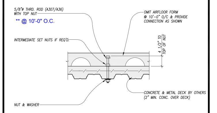
NOTE: BOLT MUST BE PLACED AT LOW POINT OF FLUTE W/ FULL CONC. THICKNESS.
