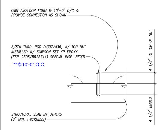
NOTE: STEPS SHALL BE TAKEN TO PREVENT THE PUNCTURING OF ANY P/T TENDON OR MILD STEEL REINFORCEMENT DURING DRILLING FOR EPOXY ANCHORS.
